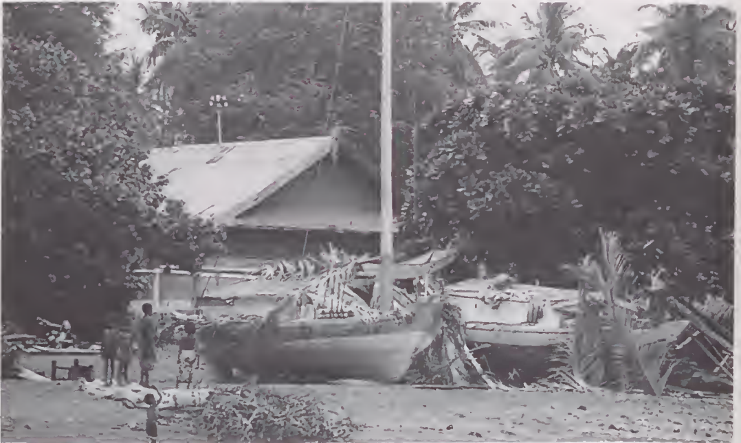
Fig. 13. Large juko with a shallow, beamy midsection.
